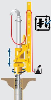
**Automatic drilling and extraction control for Single-Pass processes**
