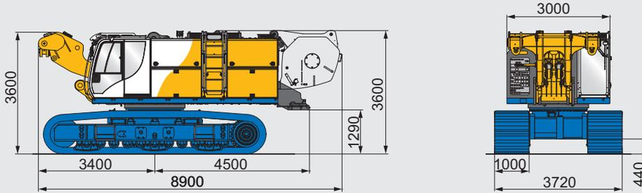
Base carrier with lower mast section
