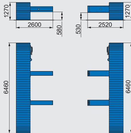
**Upper mast section with mast head**
